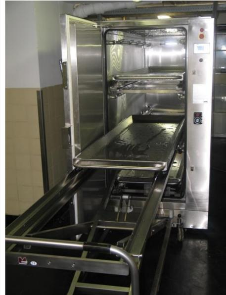
Automatic loading / unloading of the SprayCon unit
