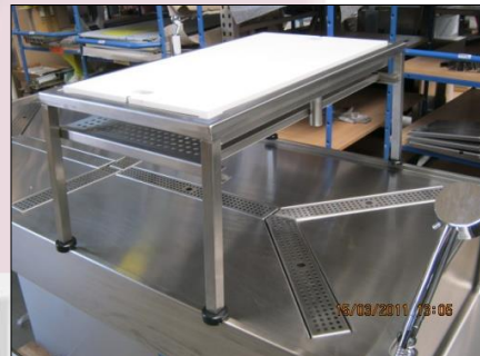
MA-3508 with special shaped worktop and integrated covered drain channels plus sliding organ grossing table with instrument tray
