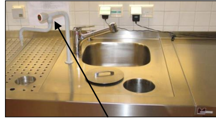
Manual formalin tap for fresh formalin mounted to a MEDIS MT Tissue Grossing Station MA-0032. Below left: waste formalin drain into 600 litres
