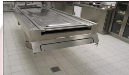
Transfer-lid opened after insertion of roll on / roll off work area (body tray)
