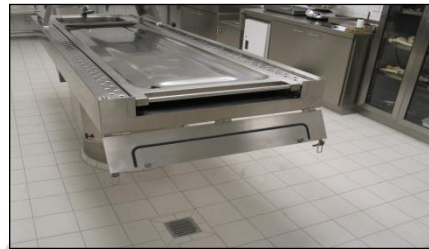
Transfer lid opened after insertion of roll on / roll off worktop (body tray)
