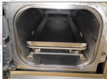
Body tray fully inserted into process chamber
