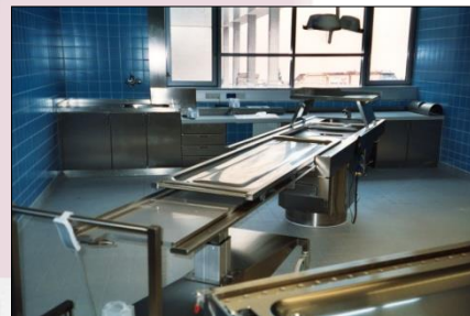
MA-2010 Universal Transporter with electr. height adj. for automatic body-transfer to / from dissecting table.
