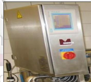
MA-1500 P.E.G. Infiltrator (version with integrated touchscreen programming)
