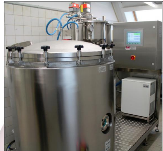
Bone fat extraction uni with DCM recycling- and bone drying module. Degreasing chamber: 1000mm AD x 900mm (H)
