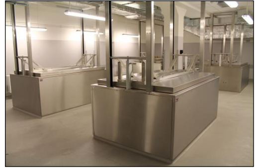
MA-1347 Preservation cuvettes for 6 cadavers each in the storage room. Inserts with cadavers are lifted hydraulically
