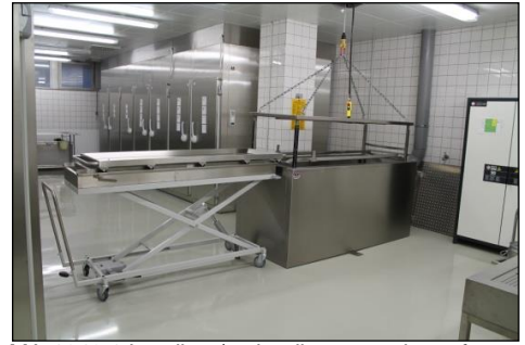
MA-1343.1 Loading / unloading procedure of a preservation cuvette in an embalming room
