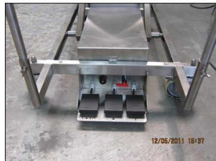
MA-1276 Body tray lifter. Electrical drive pedals (up / down / tilt)
