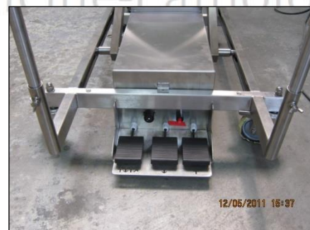
MA-1276 Body tray lifter. Electrical drive pedals (up / down)
