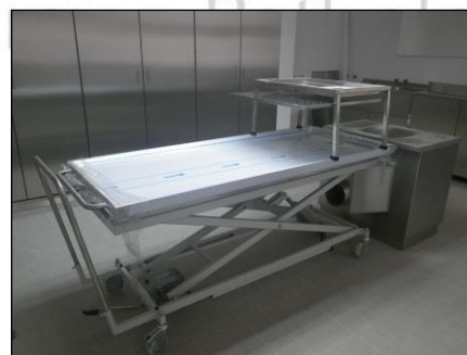
MA-1260 body lifter with body tray and organ table to be used as a mobile dissecting table
