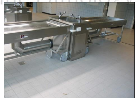
Student dissecting tables with automatic body tray transfer system and sidewall extraction docked to a double docking station
