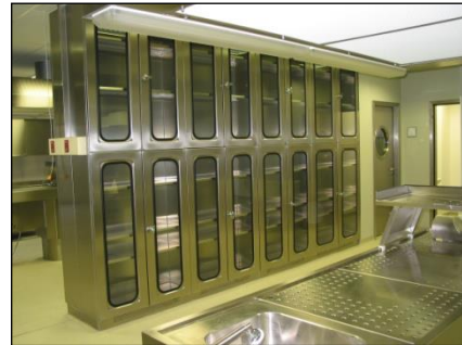
Wet specimen filing cabinet with glazed doors on both sides (room divider)
