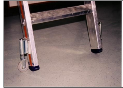
Special ladder with rollers and safety locks
