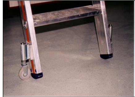
Special ladder with rollers and safety locks
